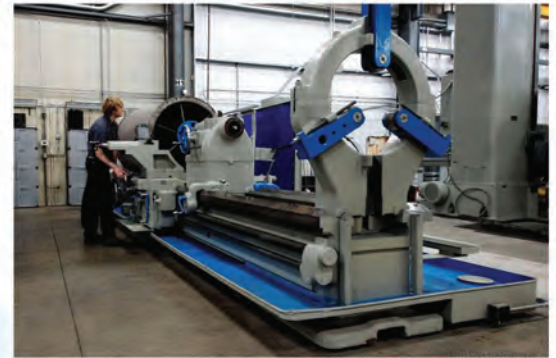
American Engine Lathe – 53" Swing, 192" Between Centers
