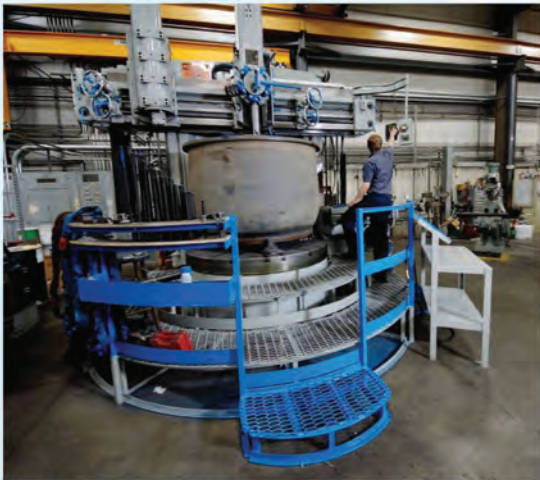
Machining VTP Diffuser
