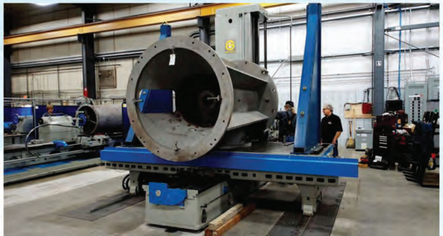
Machining Discharge Head on 5" G&L Horizontal Mill
