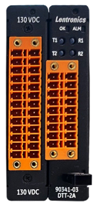
2-port Direct Transfer Trip iDSO unit (90341-03)
