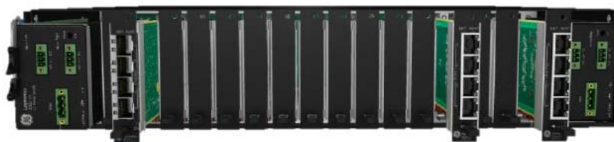
SHELF REAR SIDE WITH DROP INTERFACE PLUG-IN CARDS
