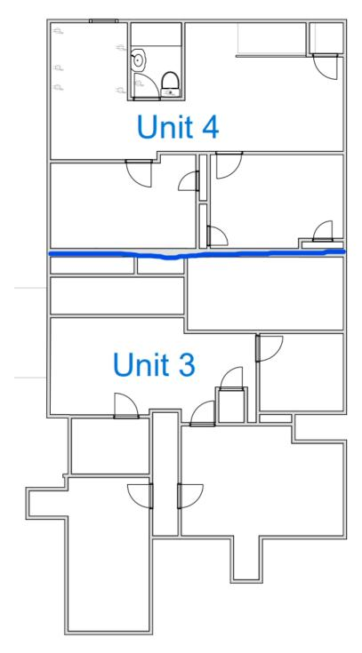
> The North side of the blue line was part of the addition in 1960 in both diagrams. The blue line is a brick wall that was the former exterior of the original structure.
