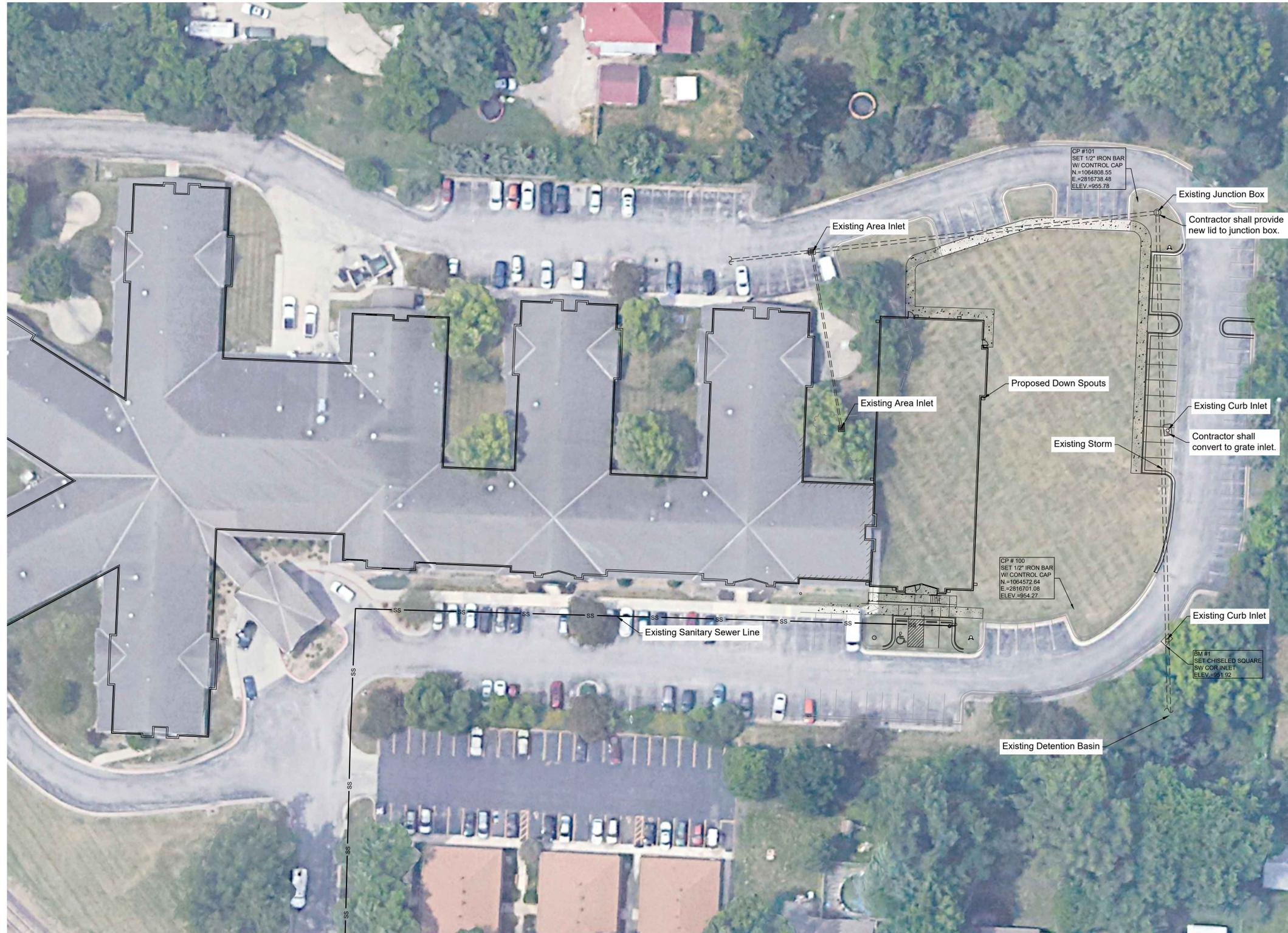
Note: Proposed down spouts are piped underground from existing building.
