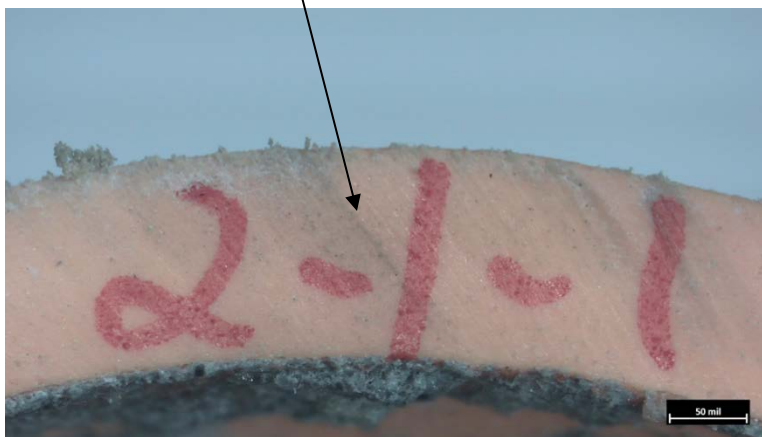
Figure B1. 36518-2-1 coating adhering to concrete, 11X magnification.
