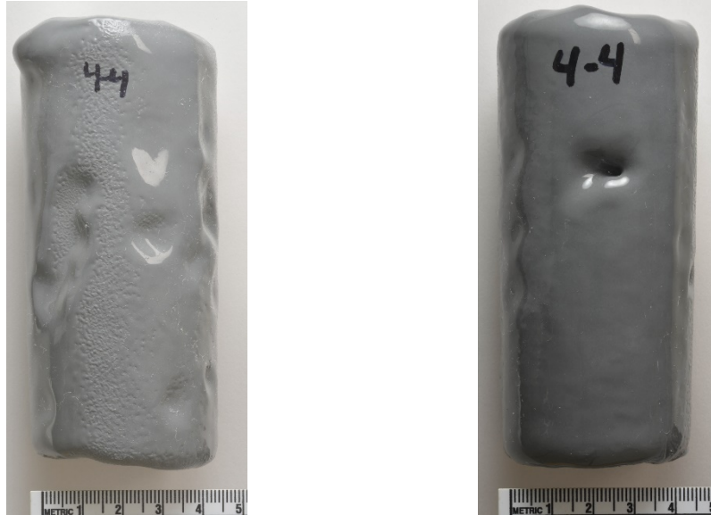
Smooth and rough sides of coated concrete.
