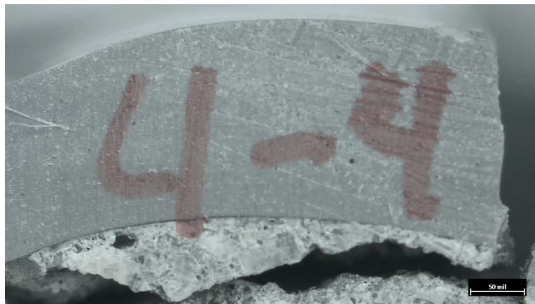
Figure B8. 36518-4-4 coating adhering to concrete, 11X magnification.
