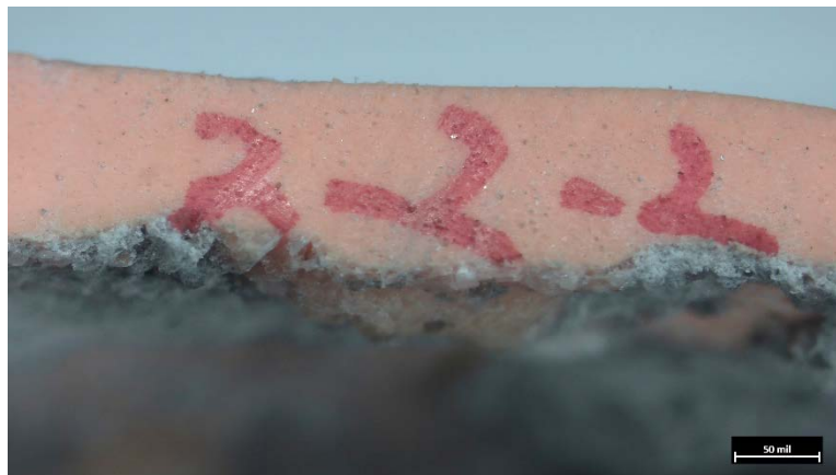
Figure B2. 36518-2-2 coating adhering to concrete, 11X magnification.
