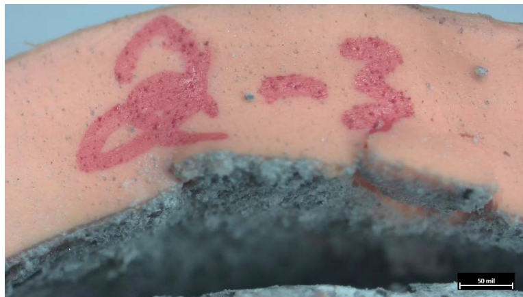
Figure B3. 36518-2-3 coating adhering to concrete, 11X magnification.
