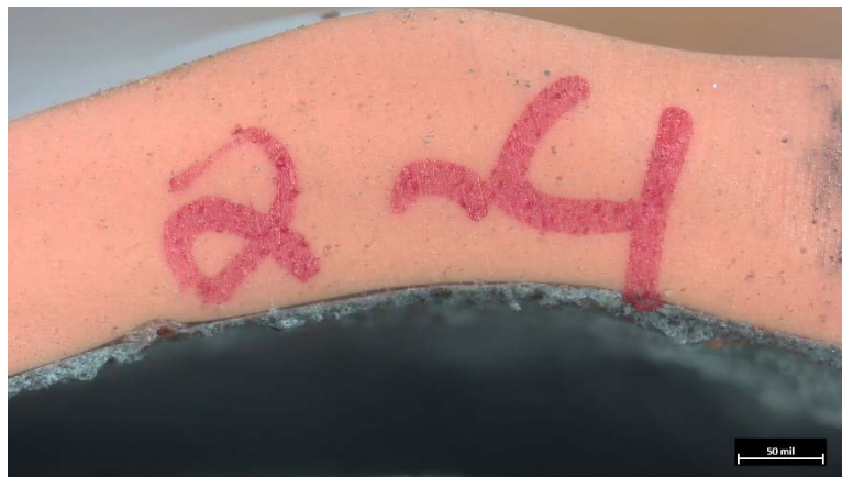
Figure B4. 36518-2-4 coating adhering to concrete, 11X magnification.
