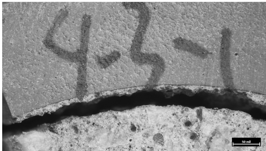
Figure B7. 36518-4-3 coating adhering to concrete, 11X magnification.
