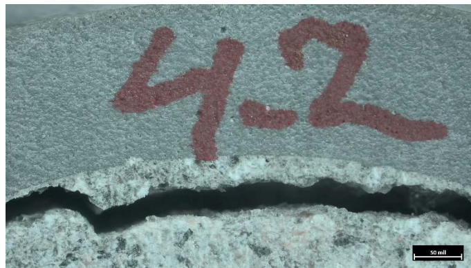
Figure B6. 36518-4-2 coating adhering to concrete, 11X magnification.
